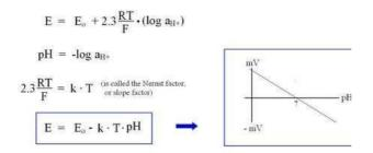
The equation  $E = E0 - kT \cdot pH$  is the potential or voltage (millivolt; mV) relation of a pH electrode. It is the equation of a straight line. The slope factor is the term "kT" and it provides the amount of change in total potential (mV) for every change in pH unit. The equation  $E = E0 - kT \cdot pH$  may be stated for any temperature. However, the slope or Nernst factor (kT) will change when temperature changes .
